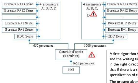
A first algorithm sought to minimize the lifts' movements, and the waiting times, by proposing the nearest lift going in the right direction. But, the first trials quickly showed that if there is a strong influx from the ground floor, the specialization of the lifts is more efficient.
